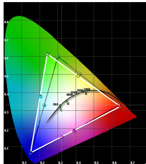
Figure 2. A typical color gamut for an evaluation-grade CRT monitor, referenced to BT.709 coordinates.
