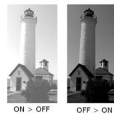
Figure 5. Using pulse-width modulation to create grayscale values.
