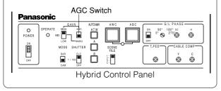
6. AGC Maximum Gain [AGC Max Gain: 6dB, 12dB, 18dB, 24dB, N/Eye L, N/Eye H] (AW-E750, AW-E655, AW-E650) [AGC Max Gain: 6dB, 12dB, 18dB, 24dB, N/Eye] (AW-E350)
