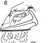
8. Plug the power plug into a household outlet and set the temperature select indicator to " **MAX** ". Impurities together with steam and boiling water will be flushed out.
