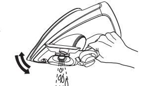
Empty the water tank immediately after using. Do not store the iron with water in it. If you empty the water tank after it has cooled, heat the iron for about 5 minutes with the temperature selector set to " MAX ".
