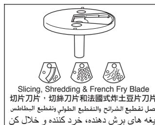
Slicing and shredding blades are used for slicing and shredding vegetables, fruits and other foods. Use "PULSE" button. Turn the switch on. At the same time press down the food with moderate force. Put in foods horizontally when using the shredding blade. French fry blade cuts potatoes into small long squares for french fries. **Always use with the blade stand.**
