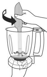
The Chutney Blade is fixed permanently. Do not attempt to remove the Blade.
