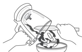
**3** After 2 or 3 minutes, tilt the Motor Housing and push the Circuit Breaker Button at the bottom surface. The appliance is now ready for resume.
