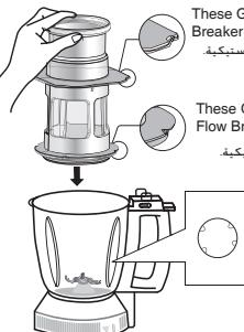
These Grooves are located at the top of Plastic Jar Flow Breaker Lines.
