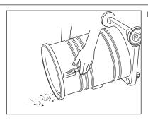
Remove the filter and empty dirt and dust.
