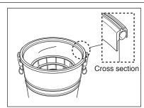
Please ensure to place the filter supporter to its original location in order to avoid filter supporter become deform which can cause dust leaking.
