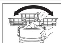
Pull the expander upward and shake it about ten times. (Never shake up and down and leave the hose connected.)
