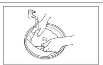
Wash the filter in water by hand. (Do not use washer or dryer.)
