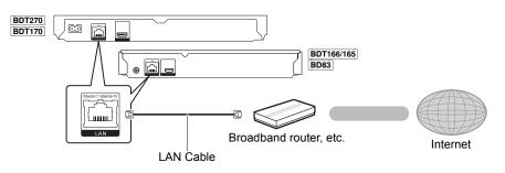
Use category 5 or above straight LAN cables (STP) when connecting to peripheral devices.
