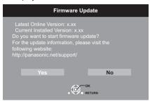
If you use BD45 or you use BD65 but downloading on this unit fails or this unit is not connected to the Internet, then you can download the latest firmware from the following website and burn it to a CD-R to update the firmware.
