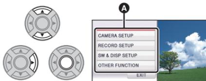
**3** Select the submenu item **B**, then press the cursor button right or press the button in the centre.
