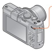
Press the rear dial to select the Exposure Compensation display
