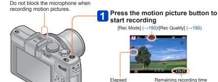
button after pressing it. Press the motion picture button again to end recording
