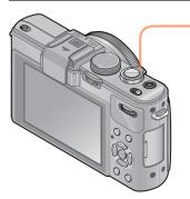
Turn the zoom lever toward the W side to display the calendar screen while displaying a 30-picture screen
