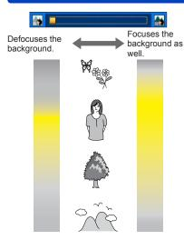
The yellow range shown in the left figure is the range for which the image is sharp.
