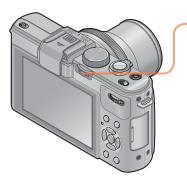
Press the [ND/FOCUS] lever to activate the ND filter
