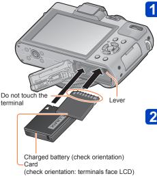
Slide the release lever to the [OPEN] position and open the card/battery door
