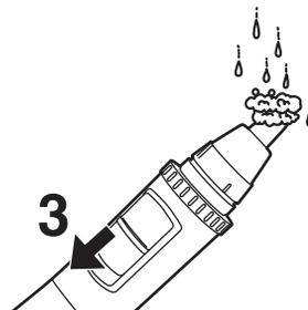
4. With the power switch still set to the “1” position, place the tip of the blade into water and rinse thoroughly.
