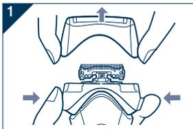
1. Press the system outer foil release buttons and lift the system outer foil upwards as illustrated.
