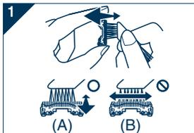
1. Clean the inner blades using the short brush by moving it in direction (A). Clean the system outer foil, the shaver body and the trimmer using the long brush.
