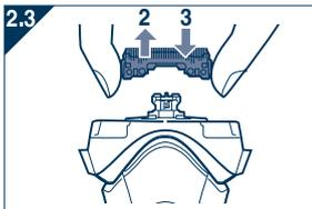
2. Remove the inner blades one at a time as illustrated.
