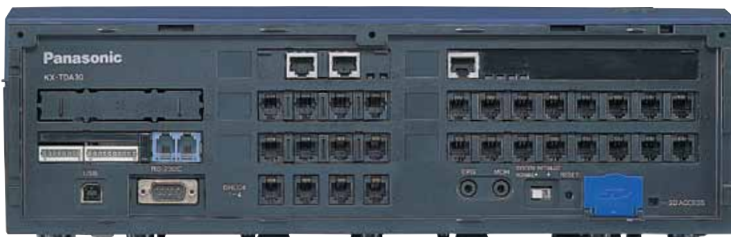
Rear view of the KX-TDA30AL. KX-TDA30AL can be rack mounted.
