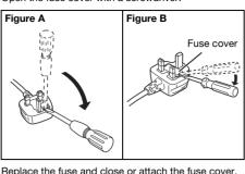
2. Replace the fuse and close or attach the fuse cover.
