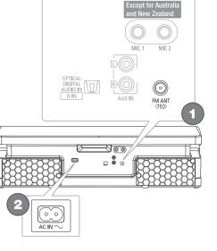
1 Connect the FM indoor antenna. Place the antenna where reception is best
