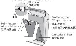
3 Remove the deodorizing filter from the poly bag. 从塑料袋中取出脱臭过滤网。
