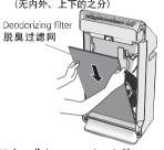
(2) Install the composite air filter. (There is distinction between the inside and outside, upper and lower) 安装集尘过滤网。
