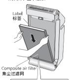
With the black side (front side) towards you and the label side up, fit it into the concave part of the main unit.
