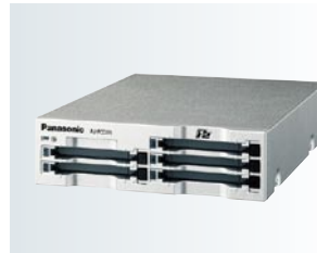
AJ-PCD35 "P2 drive" Memory Card Drive High-speed PCI Express interface.
