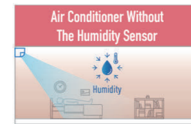
Without the humidity sensor, relative humidity increases in the room during stable operation causing uncomfortable sleeping environments.
