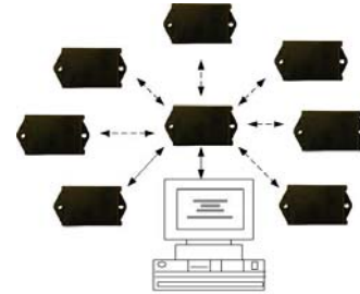
2. Temperature sensor nodes in star network topology
