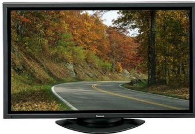
Figure 3. Allow a 1-hour warm-up cycle for any new plasma monitor before calibration.
