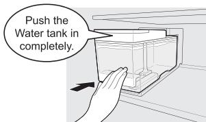
Confirm the direction of the tank and install until the tank reached the end lock.
