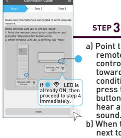
a) Point the remote controller towards the air conditioner and press the " ≈ " button once to hear a "BEEP" sound.
