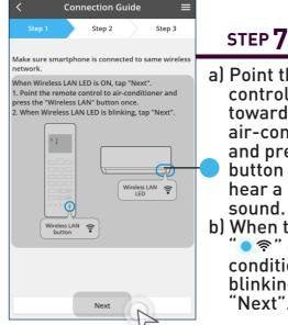
a) Point the remote controller towards the air-conditioner and press the "\varphi" button once to hear a "BEEP" sound.
