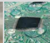
A resin-potted circuit board
