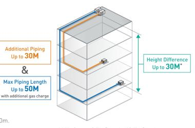
\* 4-Way Cassette, Ceiling Exposed and Ceiling Ducted (Capacity Class 17.1/20.5K Btu): 25m
