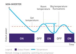
Non-INVERTER air conditioner can only operate at a constant speed which is too powerful to maintain the set temperature. This results in wider temperature fluctuations leading to wasteful consumption of energy.
