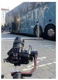
"We recorded the film in full 4K ProRes format onto SSD using Ninja V external monitor-recorders," explains De Caux. "We recorded back-up 4K to SD card internally whilst simultaneously recording to the Ninja — both for piece of mind but also to use the ProRes capability. The Ninja was linked via HDMI to the camera and triggered automatically on both internal card and Ninja V."
