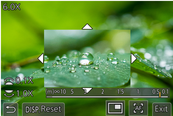
A part of the image can be enlarged up to 6 times in a windowed screen display mode (PIP (Picture-In-Picture)).
