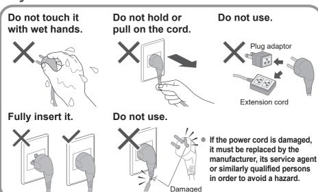
In case of failure or damaged power cord, stop use and ask the electrical technician.
