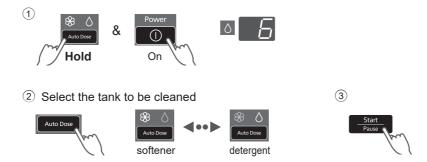
If the joint is clogged, run "Auto Dose Tank Deep Clean" function to deep clean (47-minute maintenance for detergent and softener each).
