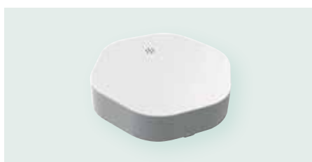
Water leakage sensor. Two sensing pads under the body activate when water is present between the two pads. Detecting the water, the sensor reports the event to the controller (and BEMS).
