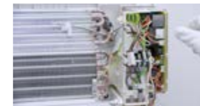
Disconnect all the connectors.
