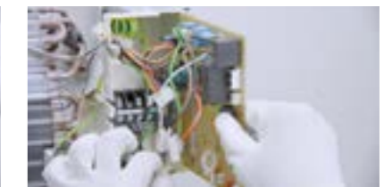
Pull out main PCB, Screw-free design makes it easy to remove PCB.
