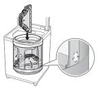
• Reverse setting cannot fix the washing board securely.
