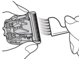
3. Brush the hairs out from between the stationary blade and the moving blade while pressing down on the cleaning lever (a) to raise the moving blade.
