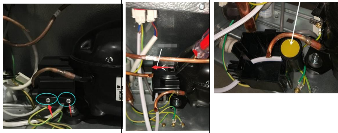
(b) Screw off the two screws as illustrated above to remove the two crimping blocks. Remove the compressor terminal box in the arrow direction, using the screwdriver as an assistant tool.
