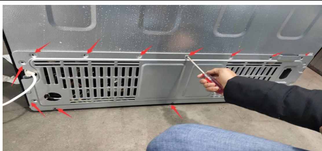
(a) Use a screwdriver to remove the nine screws on the compressor compartment rear cover.
