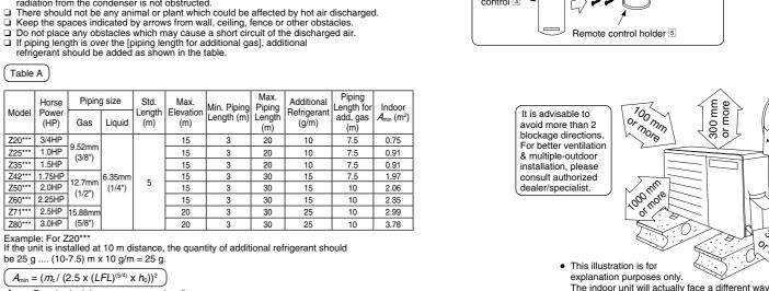
$A_{\min} = (m_c/(2.5 \times (LFL)^{(5/4)} \times h_0))^2$  $A_{\min}$  = Required minimum room area, in m<sup>2</sup>
