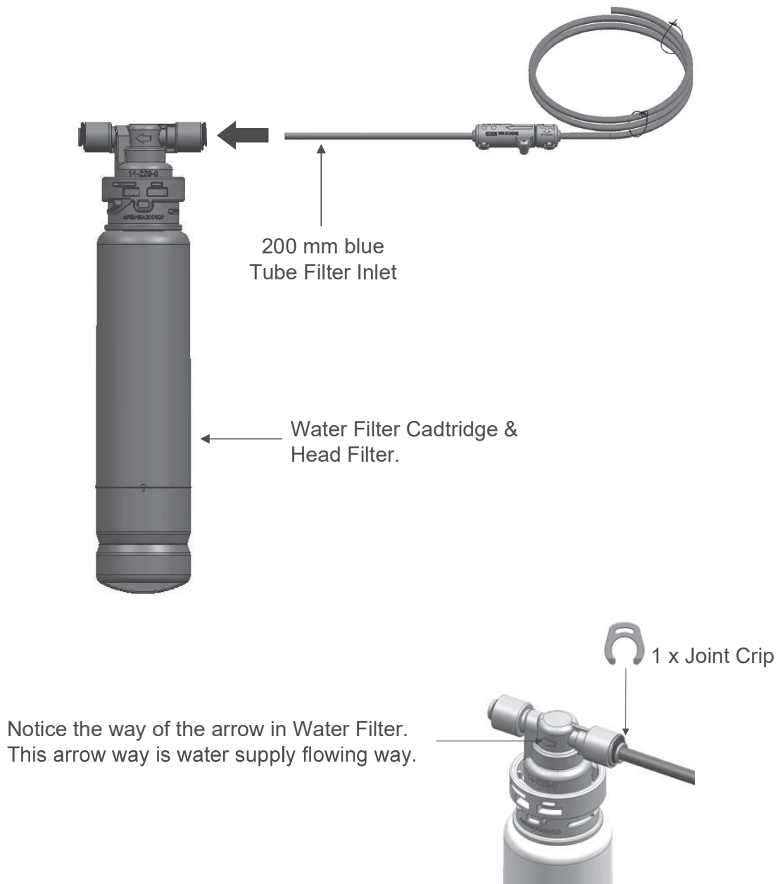
Figure 1: Connect 200 mm Tube Filter Inlet of Dual Check Valve Assembly Block with Water Filter Cartridge & Head Filter
