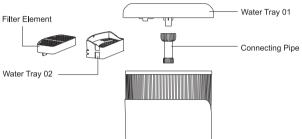
2 Put the cleaned filter element into the filter element box. (Replacing the filter element: remove the water tray 02 and replace the
