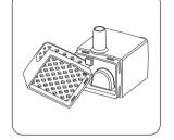
Remove panel with holding the top cover.
