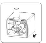
3. Remove the impeller.
