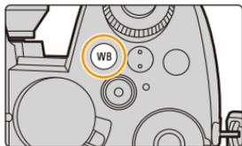
**2** Rotate the front/rear dial or the control dial to select the White Balance.
