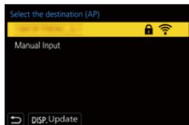
**2 (If network authentication is encrypted)****Enter the encryption key.**
