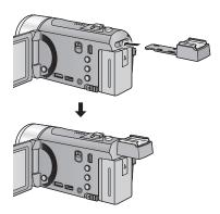
When removing the shoe adaptor, slide the SHOE ADAPTOR RELEASE lever, and remove the shoe adaptor while sliding the lever.
