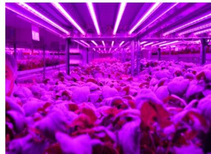
The crops will then go under LED lighting that simulates two out of seven sunlight rays necessary for photosynthesis to take place – namely blue and red light. This artificial lighting is specially tuned for cultivation in the factory where temperature, humidity and CO<sub>2</sub> are controlled. The constant environment enables stable production throughout the year.
