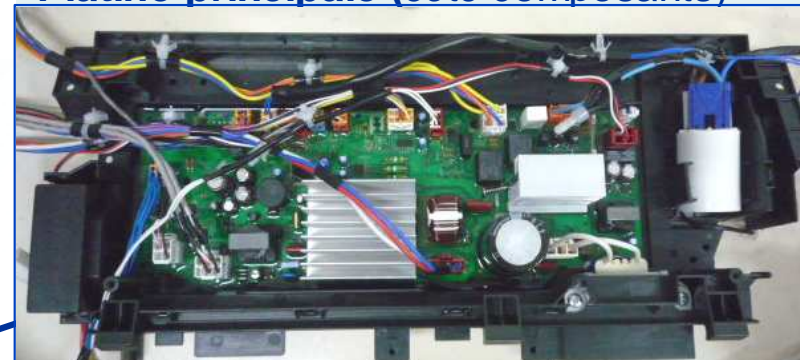
Platine principale (cote composants)
