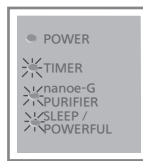
(Indication for Full load) THREE LEDs FROM BOTTOM STARTS BLINKING
