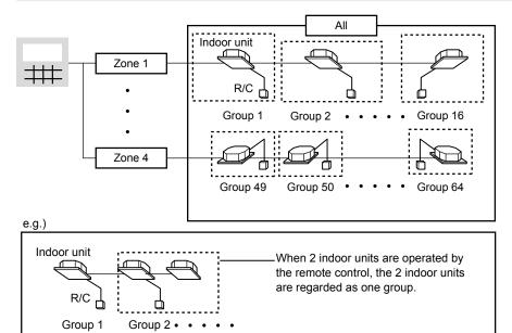
The above example shows this unit is connected as the central controller.
