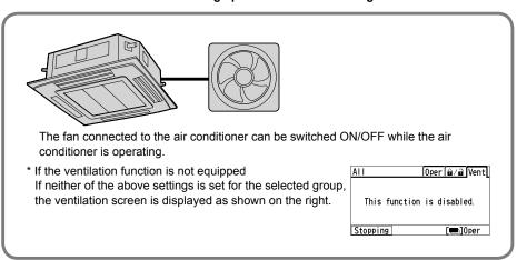
Use this setting when a commercially sold fan, etc. is connected to the air conditioner. Setting the ventilation to ON/OFF starts to operate or stops the fan. When the air conditioner is operated or stopped, the fan starts to operate or stops at the same time.
