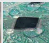
A resin-potted circuit board
