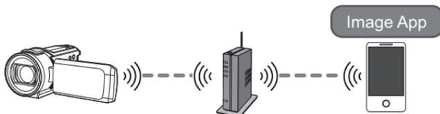
**1 Check if the wireless access point is compatible with IEEE802.11b/g/n.**
