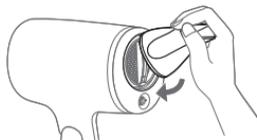
Place the nozzle to the air outlet and firmly insert it into position until locked.
