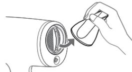
Twist and pull up the nozzle away from the air outlet.
