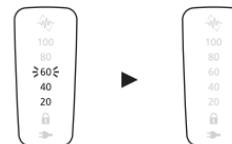
The remaining battery capacity blink and then turn off after 5 seconds.
