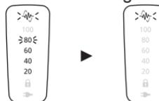
The remaining battery capacity are shown and then turn off after 5 seconds.
