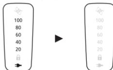
All the battery capacity lamp and ➡ will glow and then turn off after 5 seconds.
