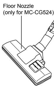
Use this function when strong suction causes the nozzle to stick to the floor, hindering movement.
