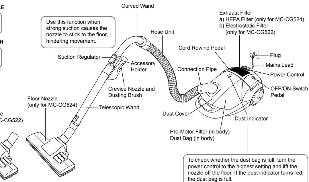
To check whether the dust bag is full, turn the power control to the highest setting and lift the nozzle off the floor. If the dust indicator turns red, the dust bag is full.
