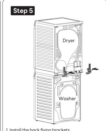
1. Install the back fixing brackets (both left and right).
