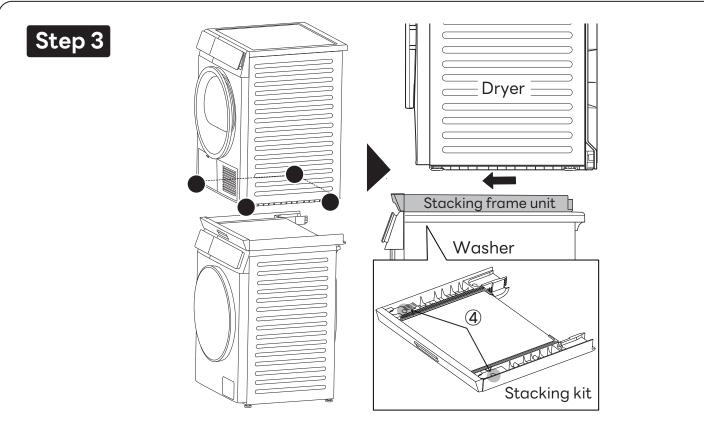
1. Lift the dryer by two people and align the front legs of the dryer on the Stacking kit at ④ as shown
