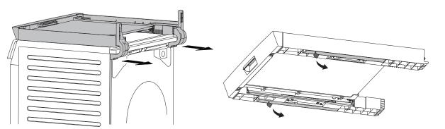
3. Remove 2 screws on the washer and remove the back fixing brackets of the washer. Remove the double-sided tape under the stacking kit.
