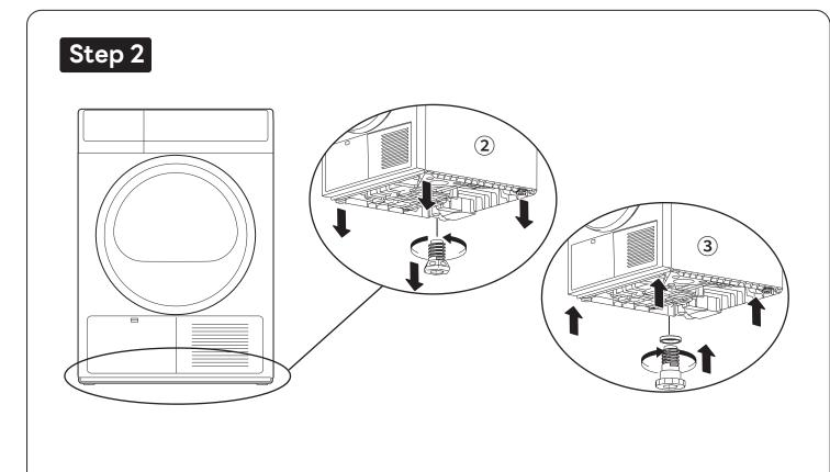
1. First remove 4 legs of dryer at ② as shown in the figure.
