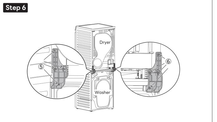
1. On the both sides, fix 4 screws in the accessories at ⑤. 2. On the both sides, fix 4 screws at 6.
