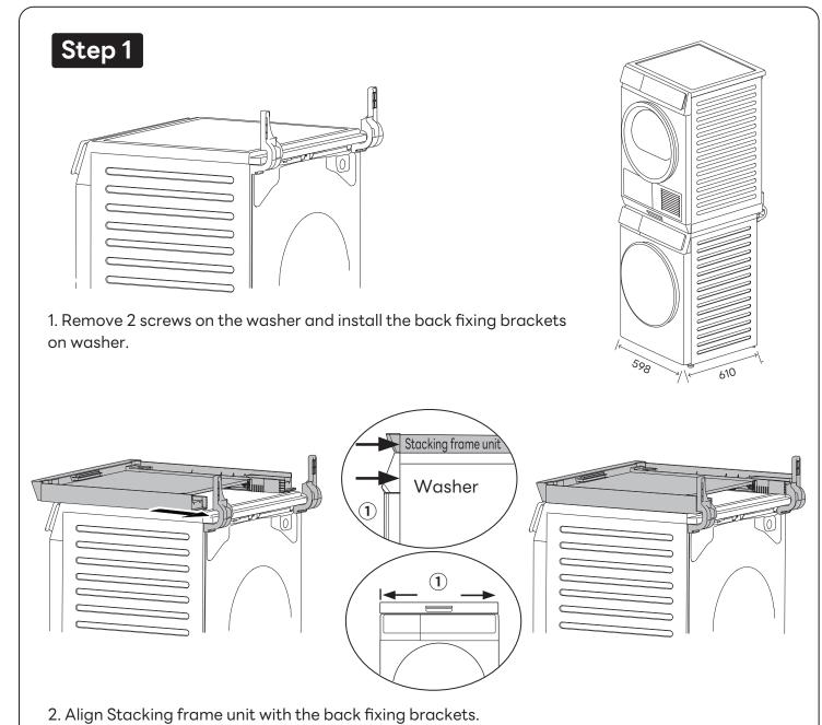
Make it centered on the top board of the front load washer and aligned on both sides at ① as shown
