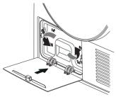
2. Turn the snap-close counterclockwise to the unlocked position.
