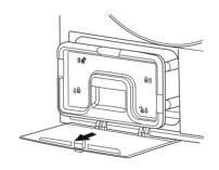
5. Push the handle assembly back. Turn the snap-close anticlockwise to the locked position. Close the heat exchanger cover on the lower part of the dryer.
