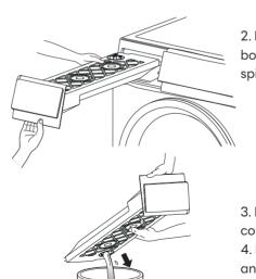
2. Hold the rear part of the condensed water box and take it out carefully to prevent water spillage.
