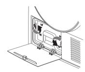
4. Clean the surface of the dryer heat exchanger with a damp cloth or brush. The efficiency of the dryer can be substantially improved after removal of accumulated lint.
