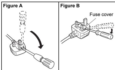
2. Replace the fuse and close or attach the fuse cover.
