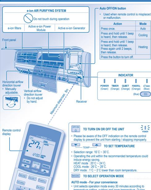
Unit selects operation mode every 30 minutes according to temperature setting, outdoor and room temperature. During operation mode selection the power indicator blinks.
